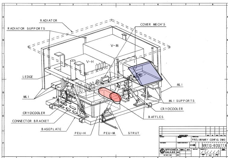
**Instrument:** VIRTIS-M-IR (1 - 5  $\mu\text{m}$ ) imaging spectrometer, Resolution~17nm, 64x64 mrad<sup>2</sup>, 256x256 pixel array
